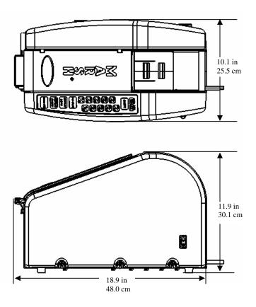
**Figure 1 – Tape Machine Dimensions**
