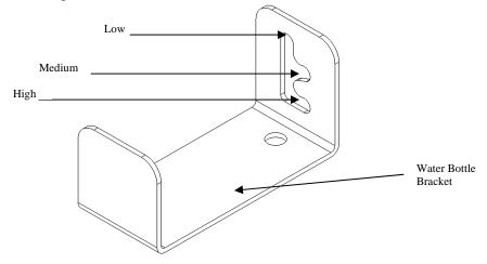
**Figure 5 – Adjustable Water Level Positions**
