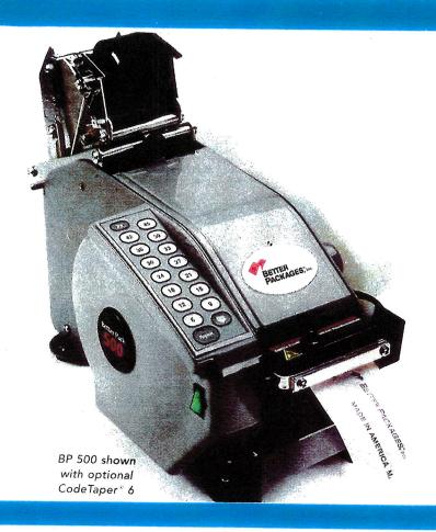
AUTOMATIC INKING The self-inking feature on the CodeTaper No. 6 eliminates the nuisance of frequent re-inking. A highly absorbent special ink roll allows long runs of dark, clear impressions between inking. The ink is transferred to an intermediate smooth rubber roller which applies it to the type roll. This procedure results in less wear on the ink roll, more even ink coverage on the type roll and consistently sharper impressions on the tape.
